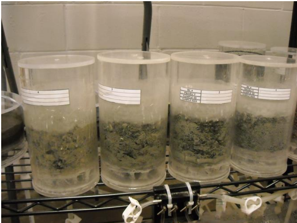
Figure 5-16: North Coal Humidity Cells in the Laboratory (Lorax, 2015)
